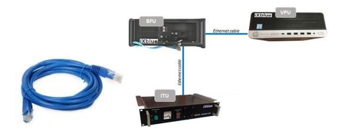
Both Ethernet cables (ITU↔BFU and BFU↔VPU) shall be terminated during the installation as per the following instructions.
