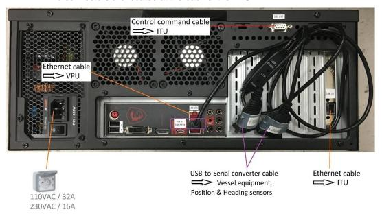
Figure 2 - BFU back face and connections
